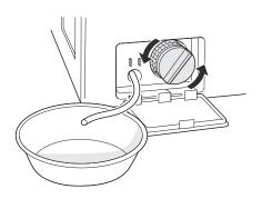
Clean the pump filter and opening.
