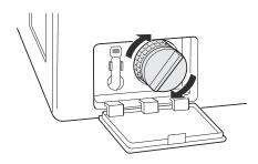
**8** Close the drain pump filter cover.
