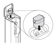
Press the battery down into the compartment.
