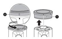
Grip the exhaust filter cover 3 and the exhaust filter **1** using both hands and rotate the exhaust filter cover while pressing the **PUSH** button in order to separate it from the exhaust filter.
