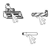
Slide the brush back into the nozzle and rotate the cover back into place. Turn the cover lock clockwise to lock the cover.
