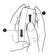
**10** Insert the clean, dry pre-filter and rotate the exhaust filter to the locked position 6 to reassemble it on the product body.
