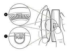
Push to insert the exhaust filter cover **3** into the exhaust filter **1** and rotate it to reassemble it and prevent it from falling out.
