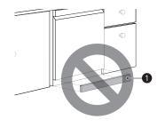
8 Remove the protective film from the door, if present. Leaving the film on may cause discoloration or condensation on the door.
