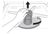
**3** Clean the filters with a soft brush under running water. Reassemble the filters before reinstalling them.
