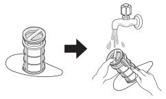
4 To replace the assembled filters, position the spray arm so the wider vee is toward the front. Fit the filters back into the filter holder and secure them by turning the inner filter clockwise until it clicks into place.
