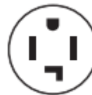
4-wire receptacle (14-30R)
