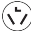
3-wire receptacle (10-30R)
