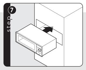
Slide cavity assembly into the cabinet opening.
