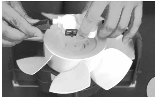
Fig 6. ... gently pull one of the motor assembly arm 1/8 inch ...
