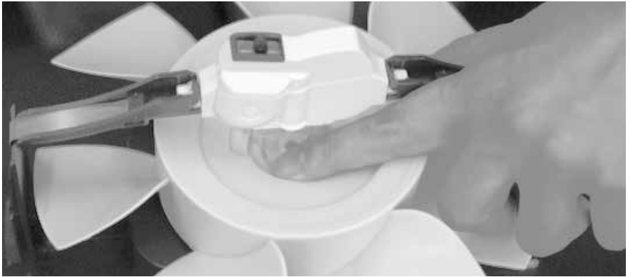
Fig 4. ... Push the coupling down ...
