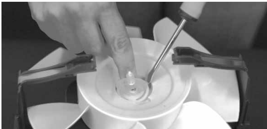
Fig 7. Remove the locking ring ... prying it up using a small screwdriver ...
