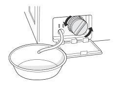
**5** Clean the pump filter and opening.
