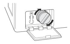
**8** Close the drain pump filter cover.
