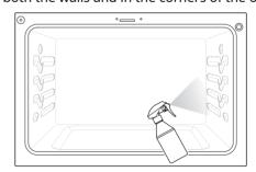
Spray or pour the remaining water (8 oz or 240 ml) onto the bottom center of the oven cavity. The indentation on the oven bottom should be fully covered to submerge all soils. Add water if necessary.
