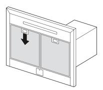
Pivot the front of the filter down and pull the filter forward to remove it.
