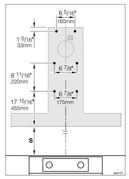
When installing a custom back wall with pre-drilled holes, please refer to the drilling distances in the drawing above (screws Ø <sup>3</sup>/<sub>16</sub>" (5 mm)).
