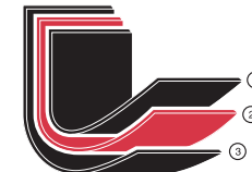
① 18/10 Stainless Steel ② Aluminum ③ Induction Stainless Steel
