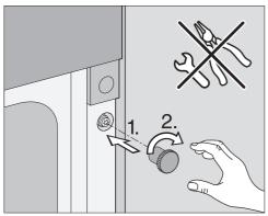
Screw the knurled nut onto the bolt by hand to fix the oven in the cabinet niche. The door may be damaged if the knurled nuts protrude from the front frame.
