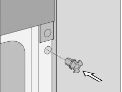
Insert the mounting aid into the hole in the front frame.
