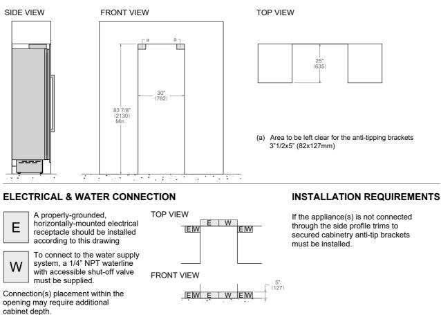
A separate circuit breaker servicing only this appliance is recommended. For installation of multiple products in combination, refer to the Built-in Food Preservation Design Guide. Dimensions in parentheses are millimeters unless otherwise specified.
