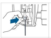
7. Secure the cable with the charging cable clip.
