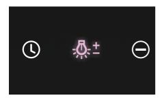
With range hood ON, press and hold Light button to adjust brightness level. You can also adjust brightness via the app.
