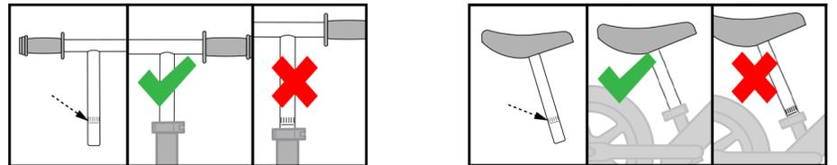
On both the seatpost and handlebar, there are minimum insertion marks. For your child's safety, insert the posts into the frame far enough so the dashed lines do not show (see diagrams above).
