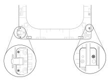
Rotate the **1** lower hinge assembly 180 degrees and install it on the right side using the two screws removed in a previous step.
