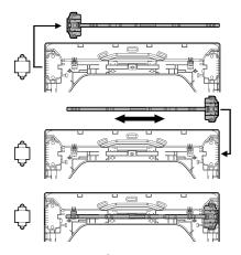
• Now rotate the **4** hinge filler 180 degrees and install it on the upper left side of the door.
