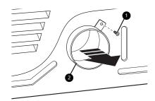
Press the adapter duct **3** onto the blower housing and secure it to the base of the dryer as shown.
