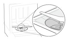
With the lower rack removed, place a level on the inside wall of the tub to check that the dishwasher is level from side to side.
