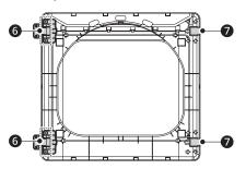
**5** With the hinges and cover caps in the new locations, remount the inner door frame onto the outer door frame with the screws removed in step 3 above.
