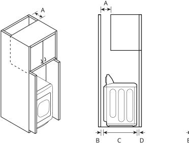
For cabinet installation with a door, minimum ventilation openings in the top of the cabinet are required.
