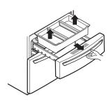
Hold both sides of the door and remove it from the rails.
