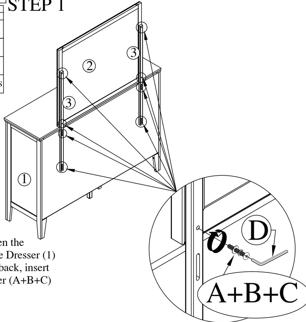
Step 1 :Attach and tighten the Mirror Support (3) to the Dresser (1) and Mirror frame (2) at back, insert JCBC (M6) With Washer (A+B+C) as shown.
