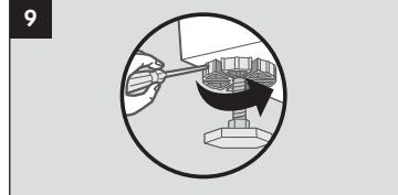
Once the washer is stabilized and does not vibrate, tighten the lock nuts on each leg of the pedestal using a flat head screwdriver.
