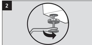
Level the pedestal with a wrench, adjusting all four legs as necessary. Use a level to make sure that the pedestal is level side to side and back to front. Do not tighten the locknuts above the feet at this time.
