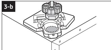
Place the feet of the washer in the outer circle of the safe landing grooves on the pedestal. The location of the safe landing groove for the washer is highlighted above.
