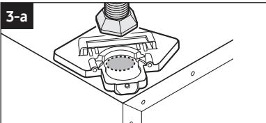
Place the feet of the dryer in the inner circle of the safe landing grooves on the pedestal. The location of the safe landing groove for the dryer is highlighted above.
