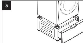
Turn the feet of the washer or dryer so that the feet are as close to the body of the washer or dryer as possible, then lock them in place. Place the washer or dryer onto the pedestal so that the feet rest properly in the clamps. See 3-a for the correct placement of the dryer and 3-b for the washer.
