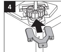
Attach a bracket leg to each foot of the washer or dryer on the pedestal, and then secure it with 4x12 screws (A).
