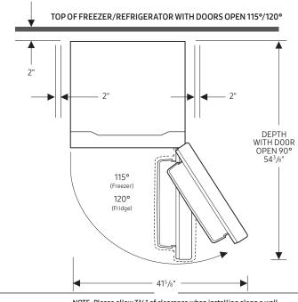
NOTE: Please allow 33/4" of clearance when installing along a wall.
