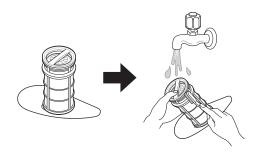
To replace the assembled filters, position the spray arm so the wider vee is toward the front. Fit the filters back into the filter holder and secure them by turning the inner filter clockwise until it clicks into place.
