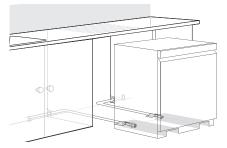
2 Smooth out or pad the edges of the hole drilled for the water supply to avoid damaging the drain hose.
