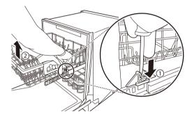
To remove the back rack supports from the rails, hold a side rail with one hand, lift the front of the rack, and firmly push the rack back to snap the support out of the hooks in the rear. Repeat on the opposite side.
