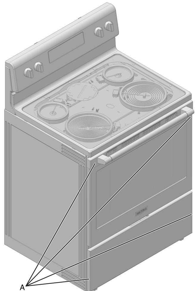
A. The model/serial/rating plate is located on the frame behind a top corner of the door or either side of the drawer.
