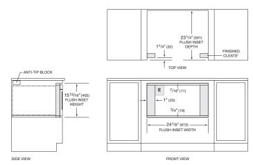
\*Will be visible and should be finished to match cabinetry NOTE: Dashed line represents profile of unit.
