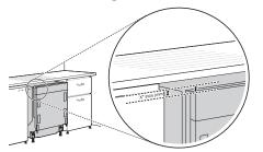
3 Using the measurement from step 2, make a mark x" up from the bottom of both rulers at the top of the provided installation template. Draw a line between the marks and trim off the top of the template at the line. Cut out the squares marked on the midline of the template so that you can see the center line.
