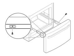
**5** Grip both sides of the drawer and pull it up to remove it from the rails.
