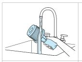
**4.** Clean cyclone with warm water and mild detergent. Let dry for 24 hours before reinstalling.
