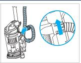
3. Attach stretch hose to back of vacuum and twist clockwise to lock into place.
