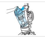
**5.** Place tank back on vacuum and press firmly until it clicks into place.
