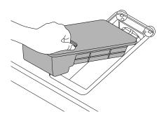
LG recommends periodic cleaning of the condenser area for thorough cleaning. To clean, loosen the screw with a Phillips screwdriver.
