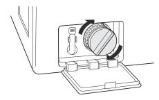
8 Close the drain pump filter cover.
