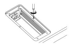
Tilt the protective grille for the condenser slightly to the left and pull it out to remove.
