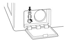
Insert the drain pump filter and twist it clockwise.
