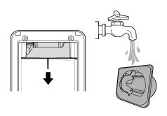
Clean the inside thoroughly with a nylon brush (not provided). Do not touch the condenser fins with bare hands. After cleaning, reassemble the protective grille and insert and tighten the screw.
