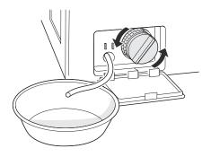
Clean the pump filter and opening.
