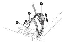
3 Rotate the hinge lever **9** counterclockwise. Lift the top hinge **1** free of the hinge lever latch **①**.
