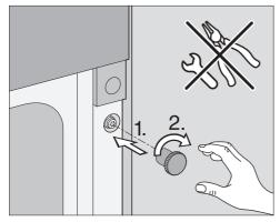
Screw the knurled nut onto the bolt by hand to fix the oven in the cabinet niche.
