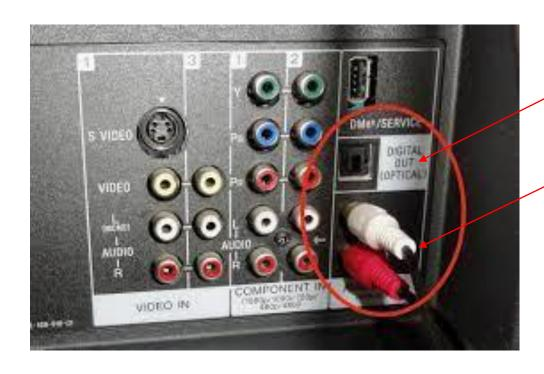
On this tv there are 2 audio output options. Digital Optical Cable or RCA jacks. Either of these options can be used to carry audio to your MotoMotion amplifier.
