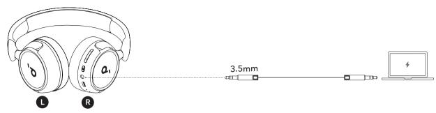
Play audio on an external device by plugging in the supplied 3.5mm AUX cable. Wired listening will automatically turn off Bluetooth mode.
