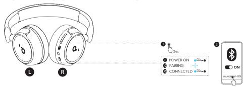
Press and hold the multi-function button for 3 seconds to power on. The headphones will automatically enter Bluetooth pairing mode when connecting for the first time. Select "soundcore H30i" on your device's Bluetooth list to connect. When pairing, the indicator on the headphones flashes blue slowly. After the pairing is successful, the indicator stays on for 3 seconds and then goes off.
