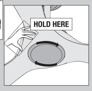
Hold the fan body stationary and rotate the light fixture clockwise to engage the locking pin.
