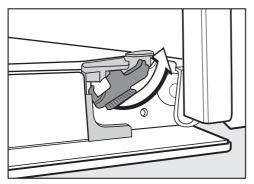
Release the locking clamps by turning them as far as they will go. You could damage the oven if you remove the door incorrectly. Do not pull the door horizontally off its retainers, as they will spring back against the oven.
