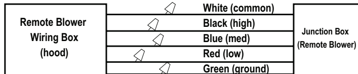
CBE-1000 / PBN-1000A: WIRING DIAGRAM
