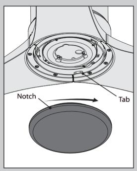
Position the notches in the outer rim of the globe or no-light cap so they line up with the tabs on the inside rim of the upper switch housing. Carefully lift the globe then rotate clockwise until it is held tightly in place by the tabs.
