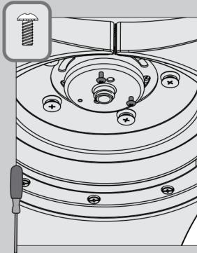
Screw two upper switch housing screws from the ≡ hardware bag halfway into the mounting plate on the bottom of the motor housing. It does not matter which two screw holes you choose.
