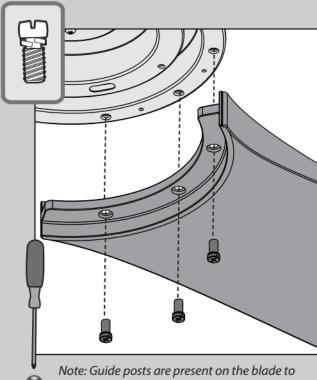
help align the blade with the motor.
