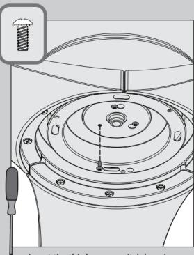
Insert the third upper switch housing screw, found in the ≡ hardware bag, into place and then tighten all three screws.
