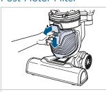
1. Press down on tab to remove Post-Motor Filter cover
