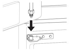
2 Fit the hinge ① over the hinge lever latch ② and slot it into place. Rotate the lever ③ clockwise and fasten the hinge.
