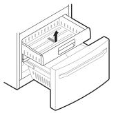
4 Remove the Durabase basket from the rails. Remove the screws from the rails at both ends.
