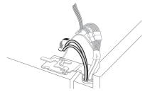
5 Hold the water supply connection and gently push in the collet ④ to connect the water supply lines as shown. Insert the tube at least 5/8 inch (15 mm) into the connector. Insert the clip on the joint to fasten the tubes in place.
