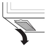
Soak grease filters in hot water and a mild detergent.
