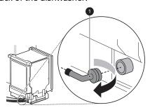
Connect the water supply tube to the elbow.
