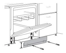
Attach a custom toe kick. If needed, use a saw to cut a notch in the top of the custom toe kick to provide clearance for the cabinet panel when opening the door.
