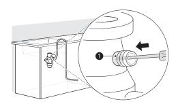
Remove the knockout plug from the disposal.
