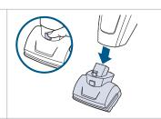
**3.** To detach, make sure machine is powered OFF. Press button on top of motorized brush and pull brush out.
