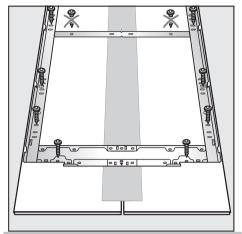
Please note: When attaching the mounting frame onto two adjacent doors (see "Front panel gap kit") screw into the thicker outer frames of the doors **only**.
