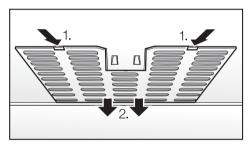
■ Unhook the filter cover, **1.** in each side of the drawer and remove them along with the filter mat downwards starting from **2**.
