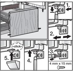
The fixing brackets are used to secure the custom door front to the bottom of the appliance door.
