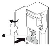
2 Open the right door and insert the combination tool ②, the crevice tool ③ and the cleaning brush ④ for storage.
