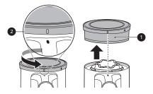
3 Grip the exhaust filter cover ③ and the exhaust filter ① using both hands and rotate the exhaust filter cover while pressing the **PUSH** button in order to separate it from the exhaust filter.
