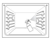
Spray or pour the remaining water (8 oz or 240 ml) onto the bottom center of the oven cavity. The indentation on the oven bottom should be fully covered to submerge all soils. Add water if necessary.
