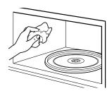
For stubborn soil, boil a cup of water in the oven for 2 to 3 minutes. Steam will soften the soil. To get rid of odors inside the oven, boil a cup of water with some lemon juice or vinegar in it.
