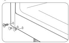
Move the Bottom Hinge to the left side of the housing, keeping the same orientation, and reattach with the two bolts and one screw. The flat screw must be placed on the exterior side of the hinge. Move the Decorative Bolt to the hole on the lower right side of the housing.
