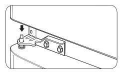
Place the Upper Hinge Pin on top of the freezer door and line up the Upper Hinge with holes on top of the refrigerator. Use the three bolts to replace the Hinge.
