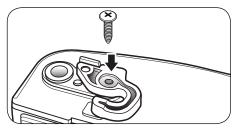
Pry off the cover on the top left side of the refrigerator to uncover the screw holes.
