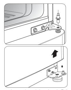
Loosen and remove the two bolts and use the Phillips head screwdriver to remove the Middle Hinge Bracket from the refrigerator housing. Set parts aside.
