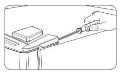
Using 10mm or 3/8 inch socket wrench, remove the three bolts and lift off the top hinge. Set parts aside
