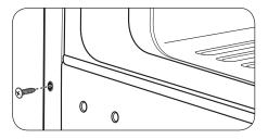
Flip the Middle Hinge Bracket, (flange will now be on top) position it on left side of the refrigerator and reattach with two bolts and a Phillips screwdriver. Place the refrigerator door down over the pin on the bottom hinge. Place the washer between the refrigerator door and middle hinge and re-attach Hinge Pin to Hinge Bracket with a ¼" socket wrench.
