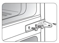
Remove the washer from the Bottom Hinge Pin. Using a  $\frac{1}{4}$ " socket wrench, loosen and remove the Hinge Pin from the Bottom Hinge. Reattach the Hinge Pin to the opposite side of the hinge.
