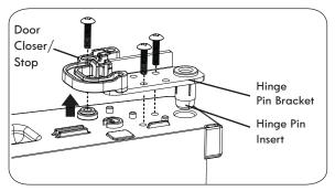
Reverse the Door Closer/Stop by flipping it over. Place it on top of the Hinge Pin Insert Bracket, and tighten both down with the screw. Tighten the Hinge Pin Bracket to the door.
