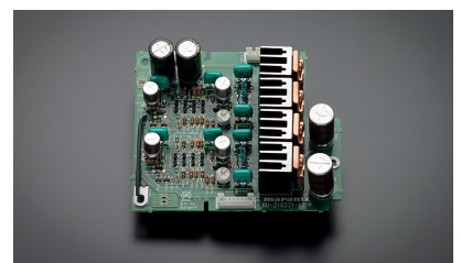
Fully discrete headphone amplifier
