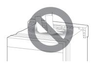
• Open the door and grab the body frame and the top front opening 2 of the tub to move or lift the dishwasher.
