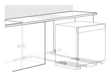
Smooth out or pad the edges of the hole drilled for the water supply to avoid damaging the drain hose.
